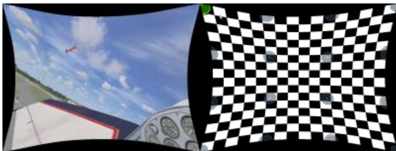
Figure 3: An example of an advanced off-axis correction
