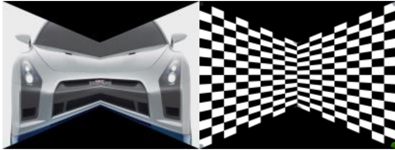
Figure 2: An example of a linear correction onto two planar walls
