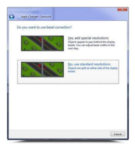
Bezel correction is use for monitor set-ups to try and minimize the software joins between the flat panels. As we are using projectors, this step is not required.
